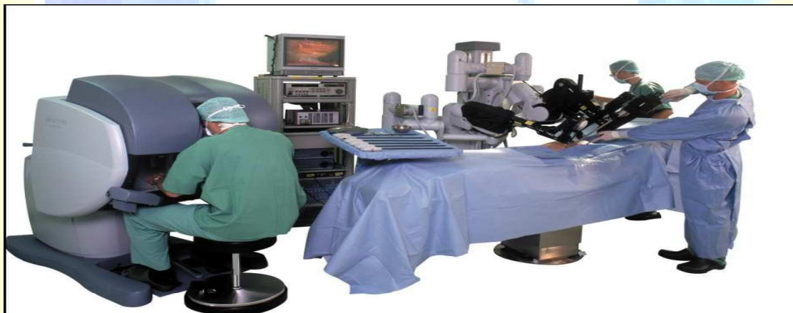
Figure 3 Master, slave and control system
